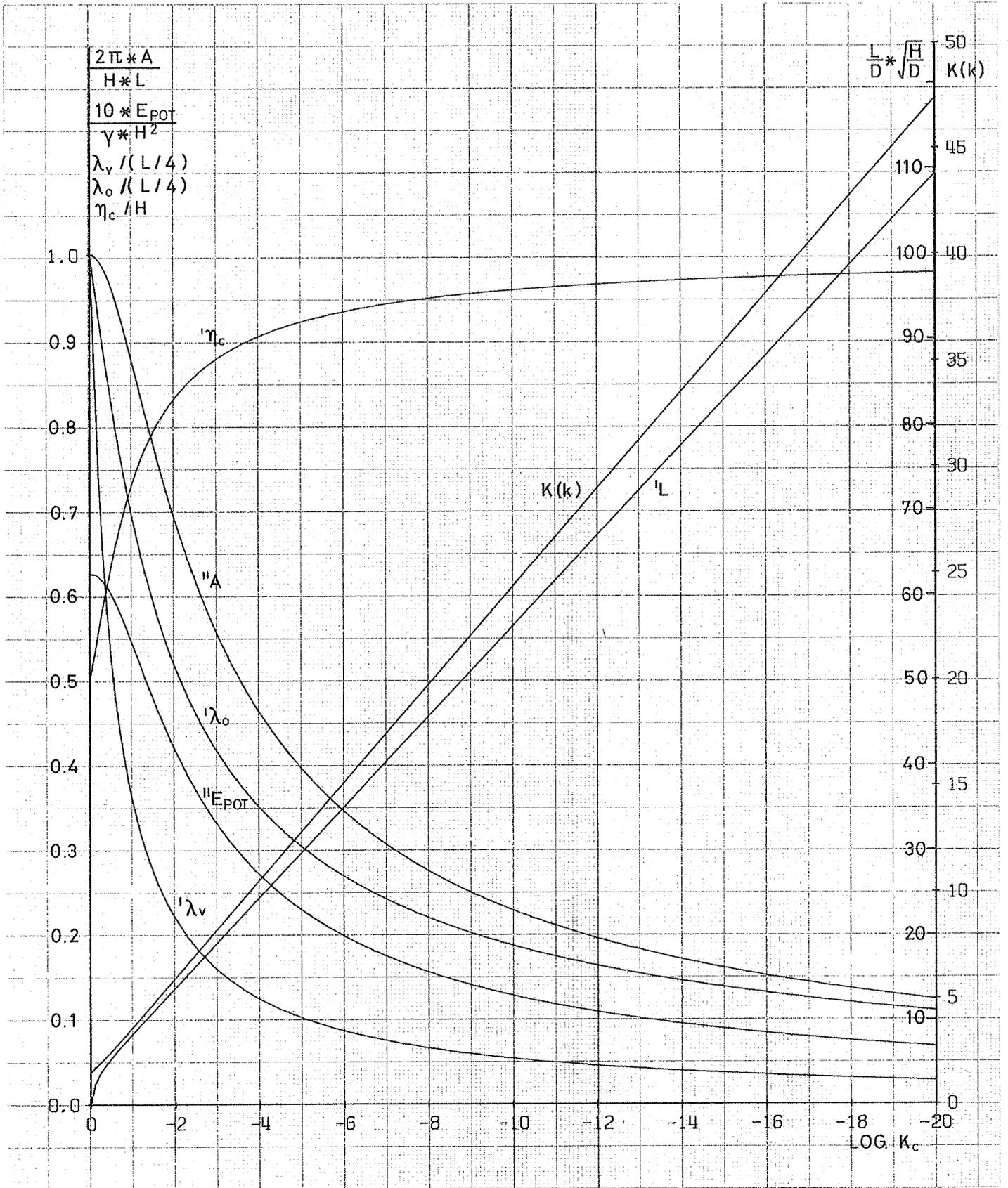
GRAPH 4. Cnoidal wave. As functions of  $\log k_c$ : wave-length, potential energy, crest-height, crest-volume, distance from the crest to the point of inflection and to the point on mean water level, and  $K(k)$ .
