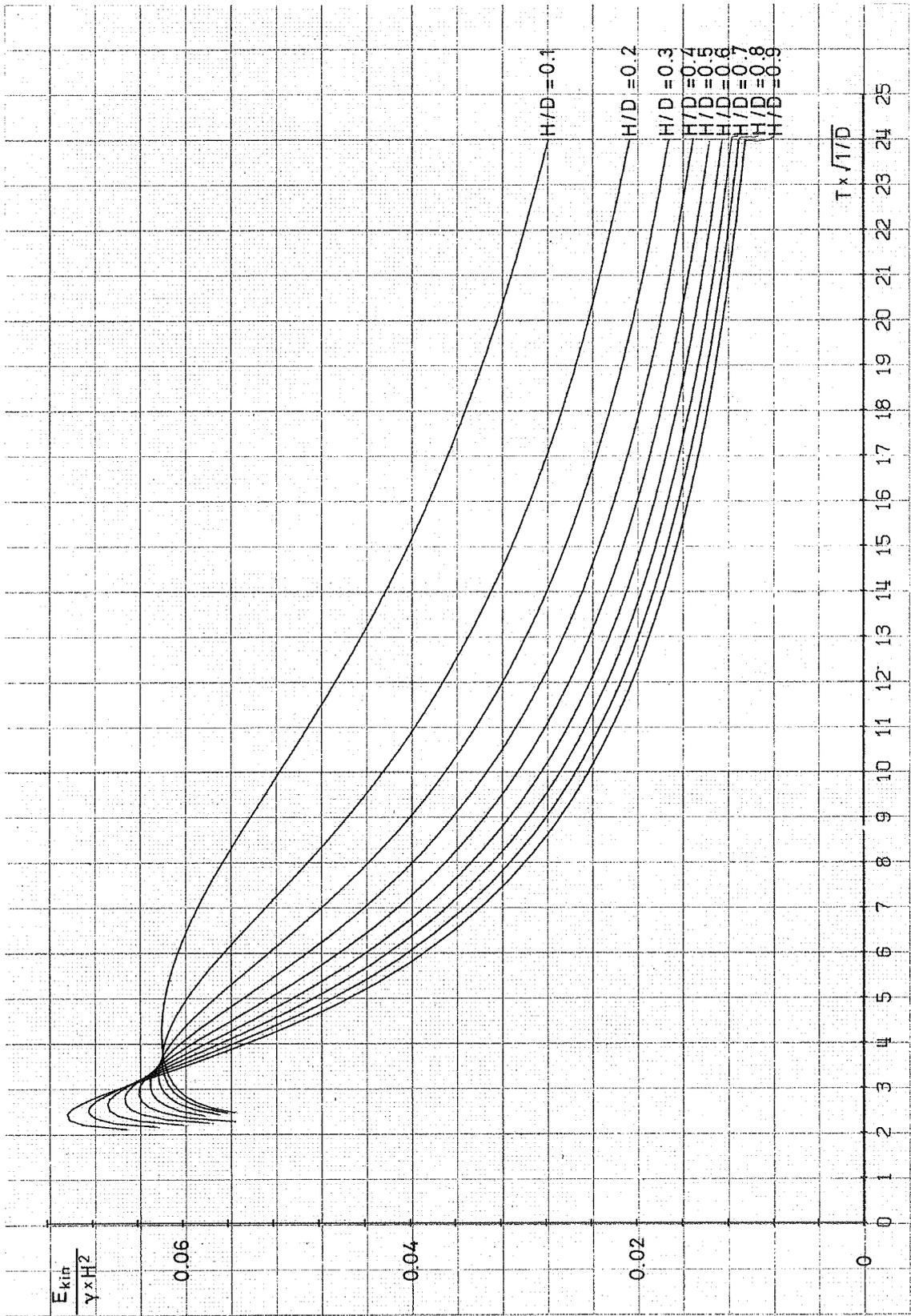
GRAPH 5. Cnoidal wave. The kinetic energy as a function of the wave-period.
