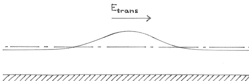
Fig. A1. The transported energy for a shallow water cnoidal wave is not just twice the potential energy.
