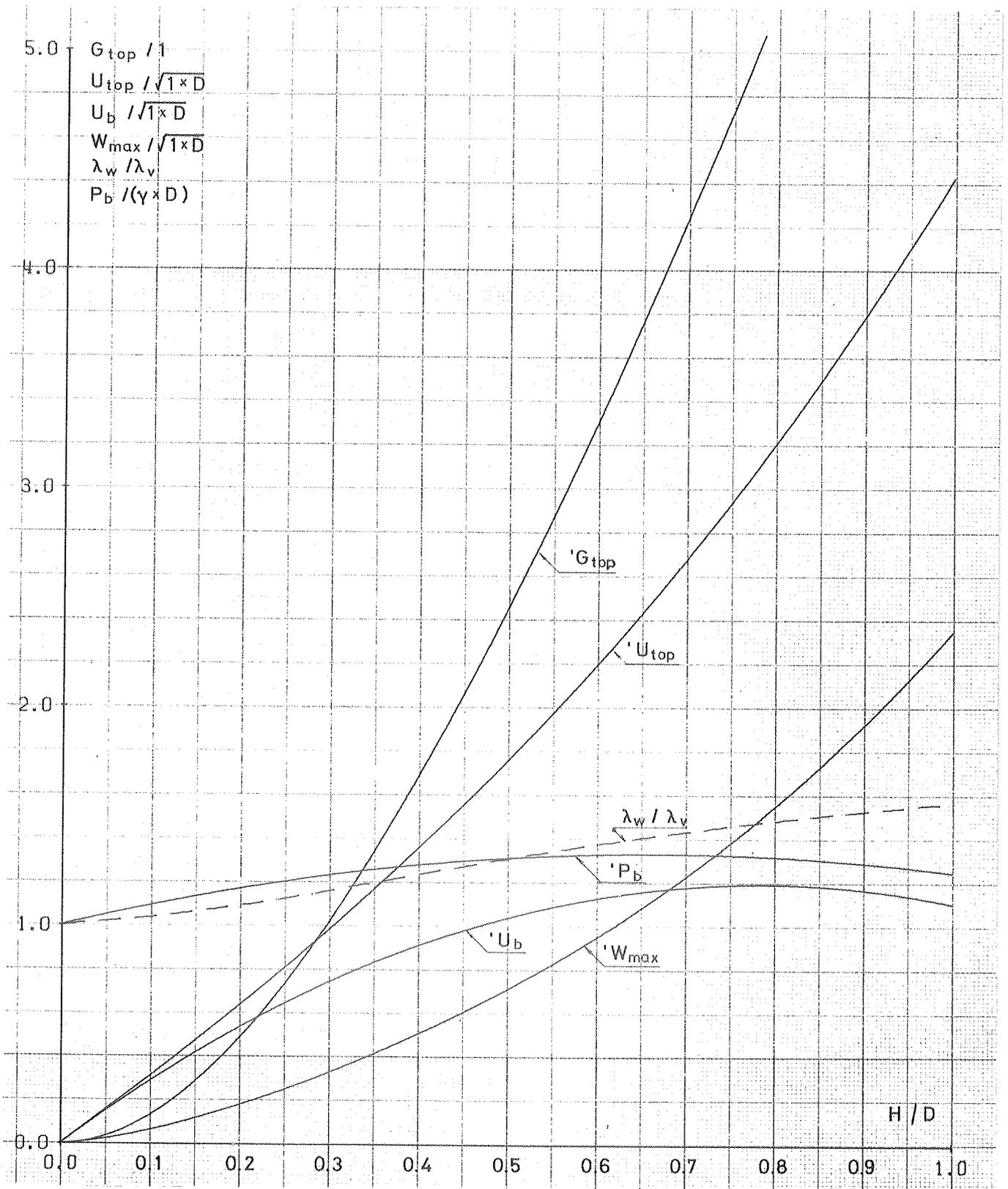
GRAPH 8. Solitary wave. As functions of the wave-height and mean water depth: particle velocities and acceleration, pressure, and the distance from the crest to the point of maximum vertical velocity.
