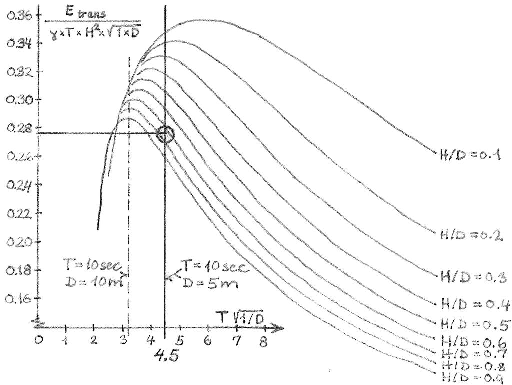
Fig. A2. Determination of the wave height. Part of graph 6.
