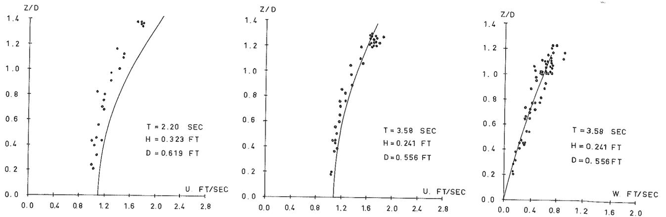
Fig.3. Comparison of theory with model tests for the maximum values of particle velocities, U horizontal and W vertical. Experiments from Mehauté et al. , reference [13]
