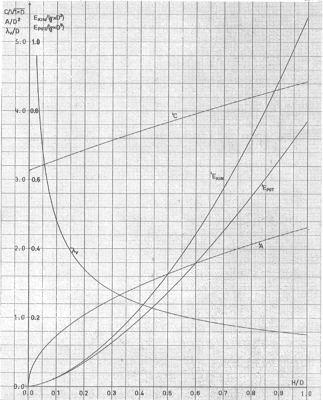
GRAPH 7. Solitary wave. As functions of the wave-height and mean water depth: celerity, kinetic and potential energy, wave volume, and distance from the crest to the point of inflection.
