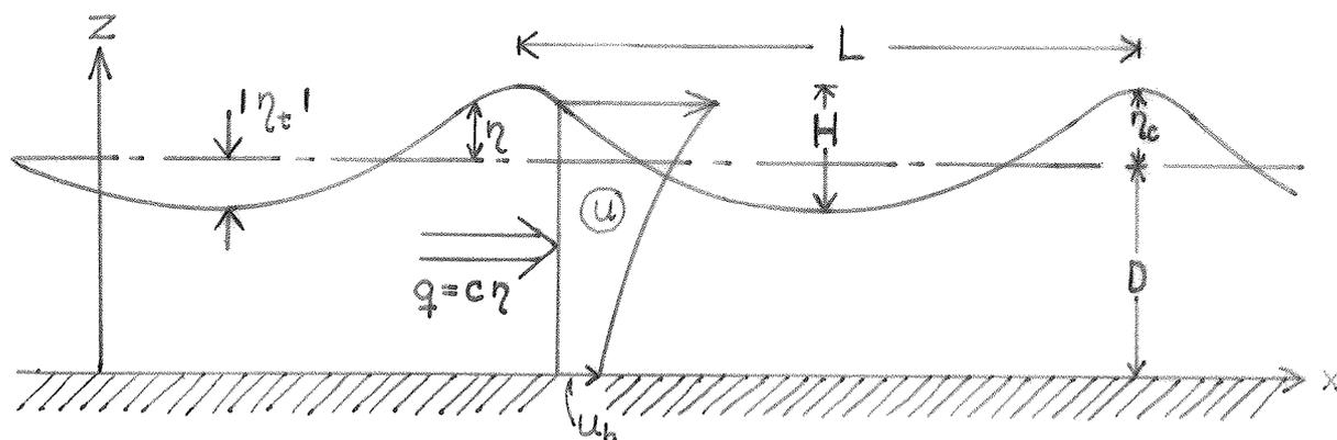
Fig. 1. In the shallow water limit the sinusoidal theory will give a parabolic velocity distribution. This can be used in second order terms to find the cnoidal theory.
