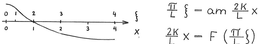
Fig. 19.  $\eta$  is still a cosine function of  $\xi$ , but  $\xi$  is an elliptic function of  $x$ , which distorts the surface profile as wanted. The result is the cnoidal wave.
