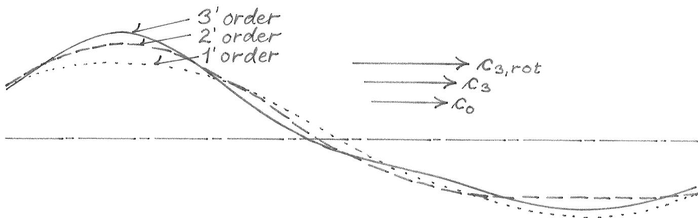
Fig. 4. The celerity of third order depends on the wave height and on the rotation of second order.
