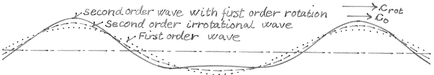
Fig. 3. Second order wave with rotation of first order magnitude (i.e. a wave on a shear stream) has second order changes in the surface profile and the celerity.
