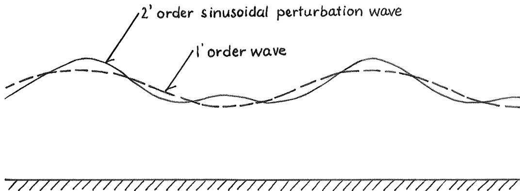
Fig. 15. The first order wave and the second order sinusoidal perturbation wave. (For deep water waves the second order wave will though never get the shown 'crest in the trough'.) The second order wave shows qualitatively how the first order profile should be changed, but a more reasonable solution than the perturbation solution should be tried.
