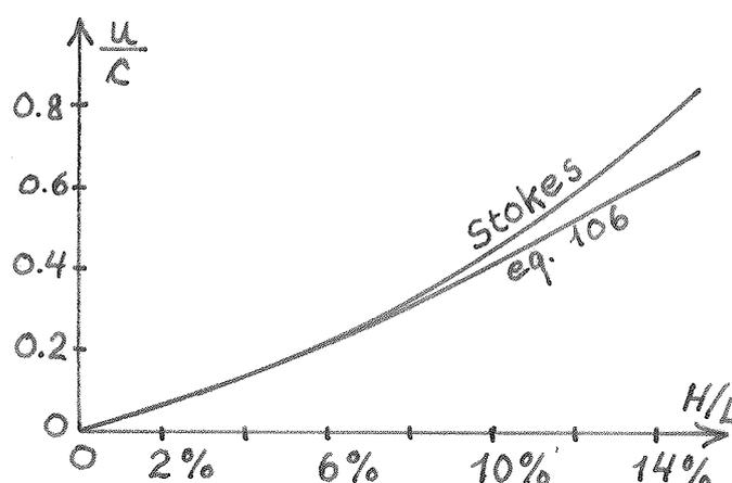
Fig. 14. The horizontal velocity at the surface of the crest for two second order irrotational sinusoidal deep water waves, the Stokes' wave and the second order sinusoidal wave of this chapter.
