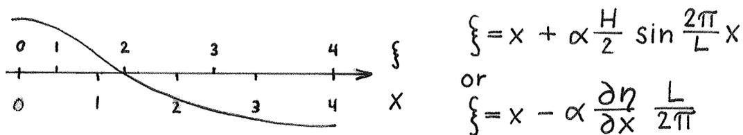
Fig. 18.  $\eta$  is here a normal cosine function of  $\xi$ , but  $\xi$  is now a function of  $x$ , which distorts the surface profile to give the wanted more narrow crest.
