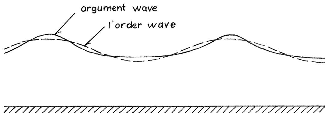
Fig. 16. By including the second order correction in the argument of the cosine function, the wave profile changes as wanted. But big changes cannot be made in this way.
