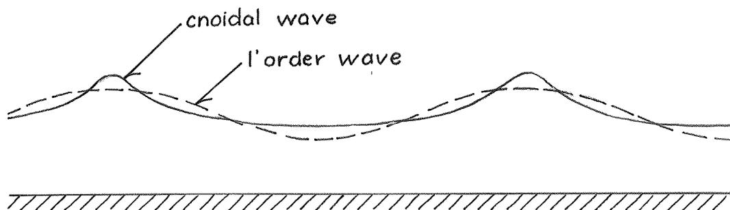
Fig. 20. If the argument of the cosine function is changed by an elliptic function to give the cnoidal wave, the changes of the surface profile can be made as big as wanted, and the wave profile will always have a reasonable form.
