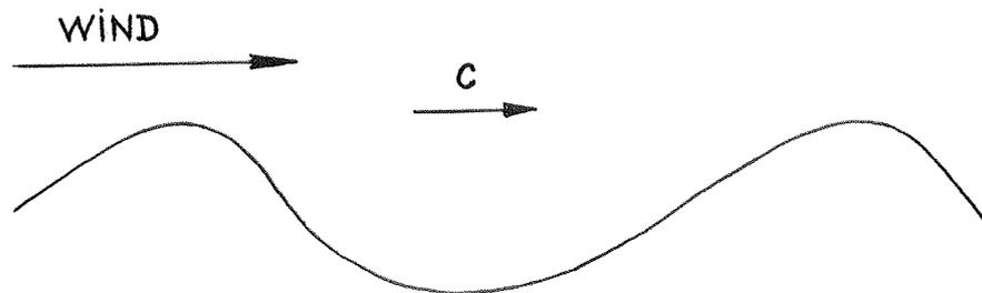
Fig. 6. During the generation of waves by the wind the pressure on the surface will not be  $p = 0$ . The result will be the asymmetrical wave.
