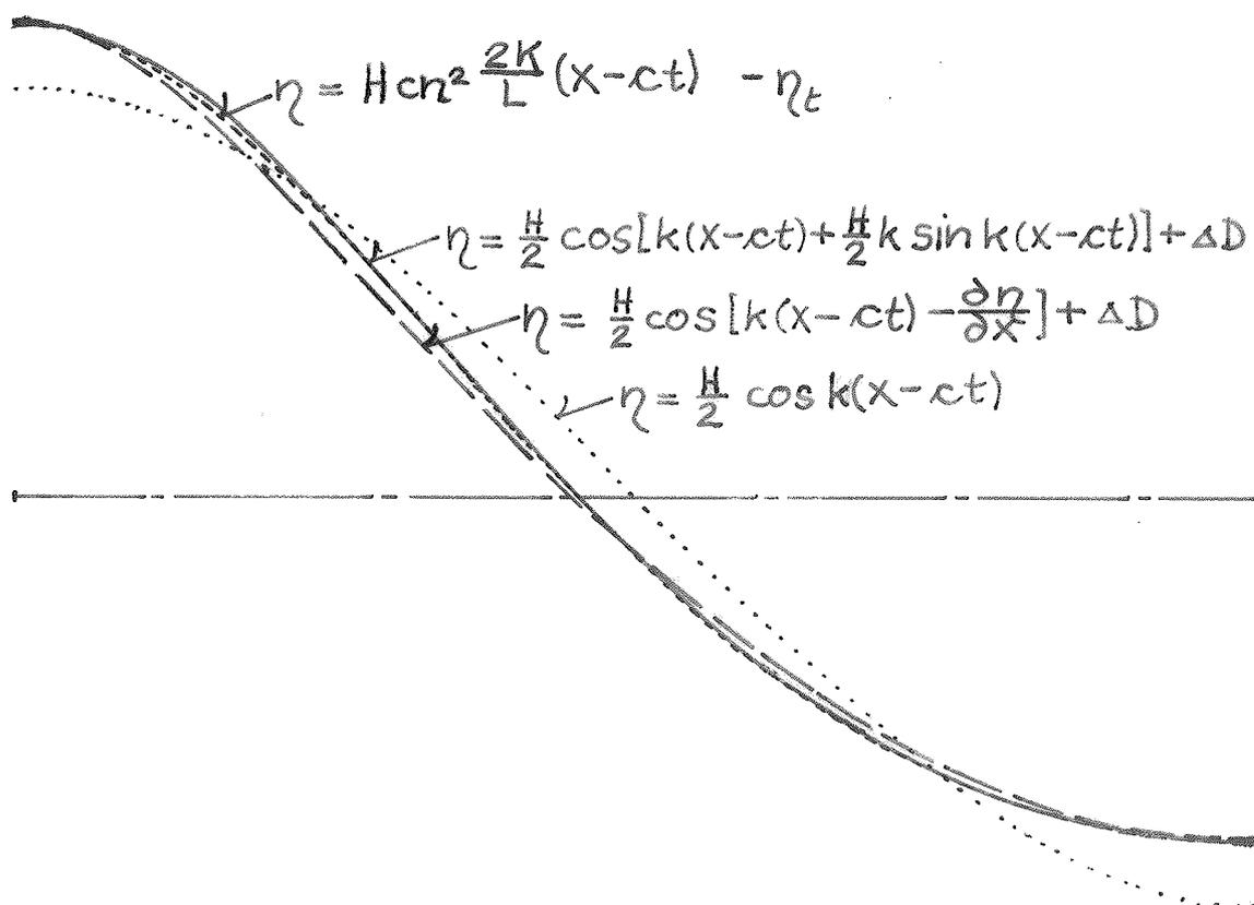
Fig. 13. Comparison of different second order waves for the deep water wave with the steepness  $H/L = 10\%$ . For infinite deep water the difference is not big. There is though a small difference between the two sinusoidal waves, and this is due to the influence of the third and higher order terms not considered in a second order theory. The second order wave above that is closest to the cnoidal wave is (incidentally) also a third order wave.
