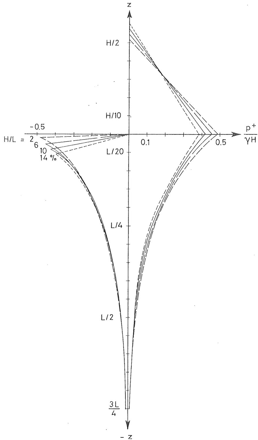
Fig. 9. Maximum positive and maximum negative wave pressure below the progressive cnoidal wave for different steepnesses:  $H/L = 2\%$ ,  $6\%$ ,  $10\%$  and  $14\%$ . Note that the unit is different below and above the mean water level,  $z = 0$ .
