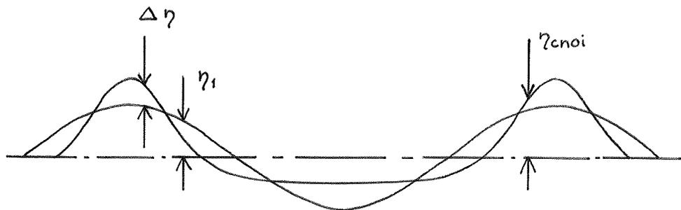
Fig. 11. The cnoidal wave is during the wave development considered to be only a magnitude of second order different from the first order wave.
