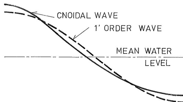
Fig. 2. Cnoidal deep water wave compared to the first order wave for  $H/L = 10\%$ . The second order waves in eqs. 16 and 17 will give the same profile. The perturbation solution from eq. 15 will be only slightly different.
