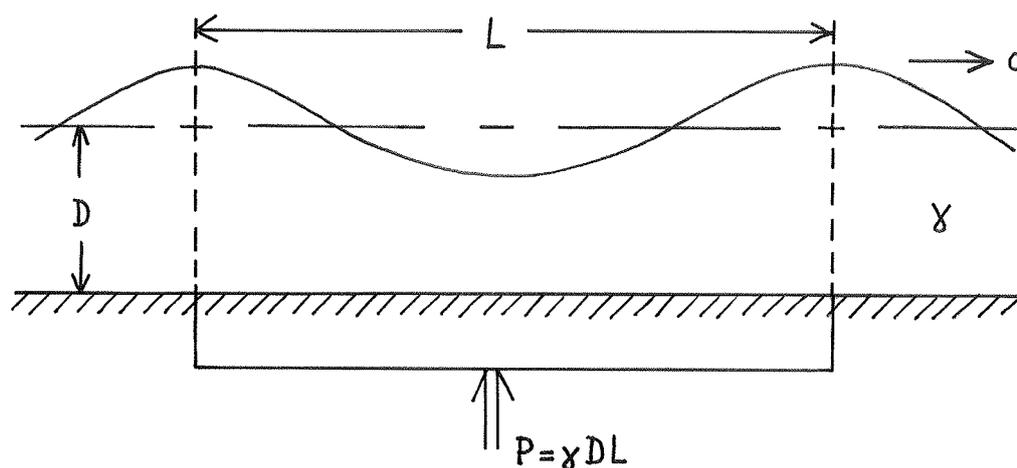
Fig. 7. At the bottom there is a dynamic boundary condition, which is as simple as shown above for the progressive wave. For progressive deep water waves it is special simple.
