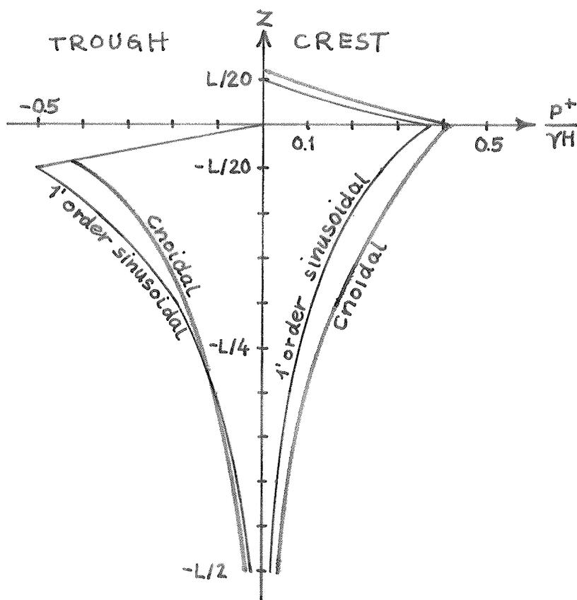
Fig. 8. Comparison of the pressure in the cnoidal wave with the pressure in the first order sinusoidal wave for a progressive deep water wave with the steepness  $H/L = 10\%$ .
