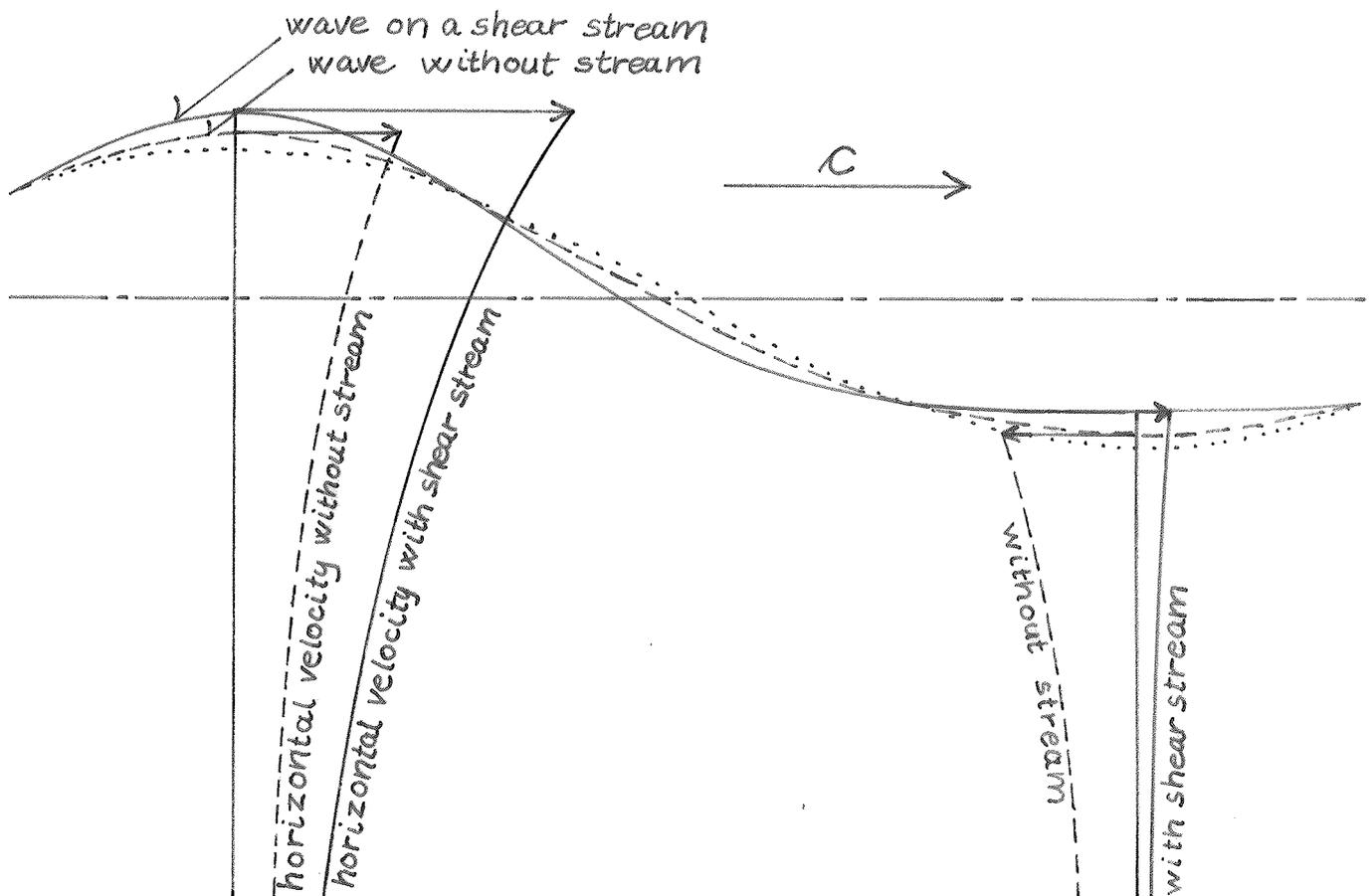
Fig. 5. Second order deep water wave propagating on a shear stream.
