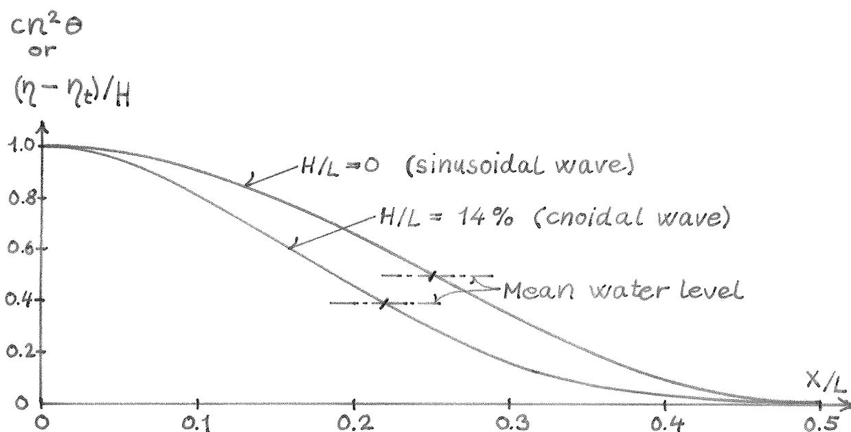
Fig. 21. The wave profile for the progressive cnoidal deep water wave of maximum practical steepness, i.e.  $H/L = 14\%$ , and the profile of the sinusoidal wave. For all other steepnesses the wave profile will be in between.
